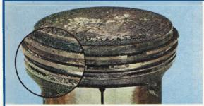
Many Motor Oils build up gummy, varnish-like deposits on vital engine parts (see piston above). A dirty engine wears out faster, needs repairs. Magnified area shows clogged, stuck rings which cause loss of power and high oil consumption.
